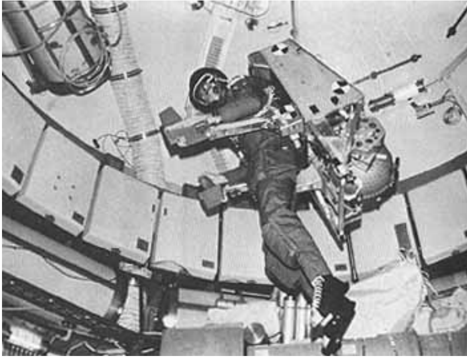
A Skylab 3 onboard photo shows astronaut Jack R. Lousma as he flew the astronaut maneuvering unit in the forward dome of the space station while in Earth orbit.
