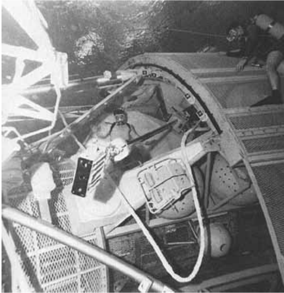
Activities at MSFC on 5 January 1972 during a simulation of film retrieval from the Apollo telescope mount in the MSFC Neutral Buoyancy Tank.
